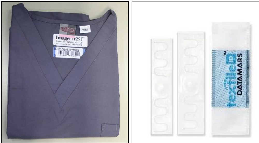
FIG. 1: Placement of the tag in a shirt (left). UHF LaundryChip (right).
